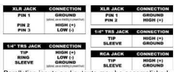
Paralleling inputs and outputs may be accomplished by using any of the 3 connectors.
